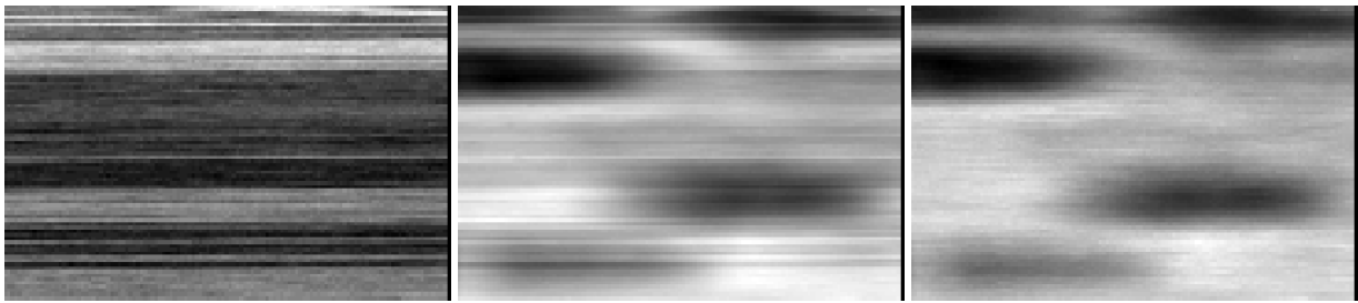
FIGURE 5. An example of a flat-fielded C-scan taken of a 0.4 mm thick uni-weave carbon fiber fabric. The left image represents reference amplitude levels taken before the waveform traverses the sample. The middle image represents amplitudes taken after the waveform passes through the material. The image on the right is the through-transmission C-scan values divided by the normalized flat-field values.
